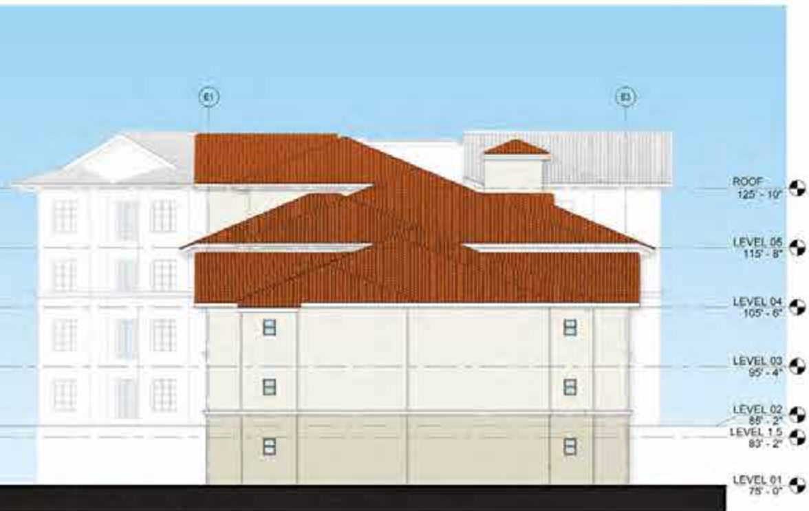
2 BUILDING 2 ELEVATION - SOUTH 3/32" = 1'-0"
