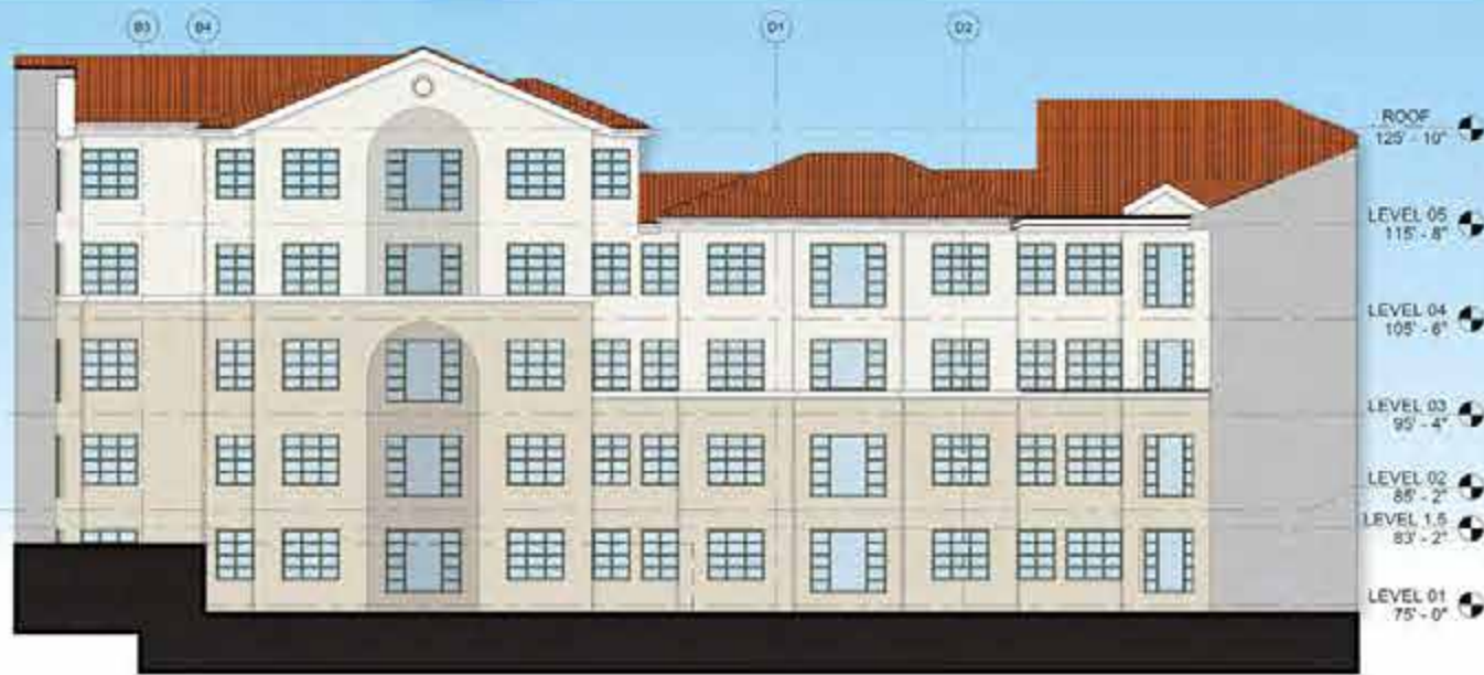
2 BUILDING 1 COURTYARD ELEVATION - EAST 3/32" = 1'-0"
