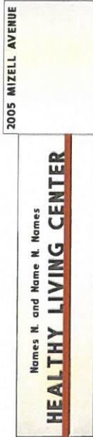
1 SAMPLE CONCEPT - SITE SIGN - GROUND SOURCE ILLUMINATION PROJECTING AND ANGLE BRACKETED FLAT CUT LETTERS - DAY TIME VIEW SCALE: 1/4" = 1'-0"
