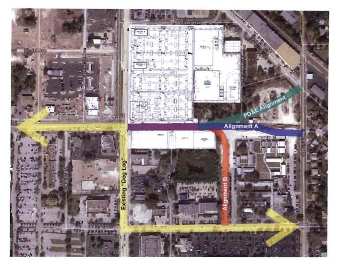
**"PD&E" alignment:** The preferred alignment from the 2004 FDOT study shows Lee Road extending east along the Cherokee Avenue right of way then curving northward to a reconfigured Denning/Solana intersection using the school board property. The cost to construct this extension was originally estimated to be \$11.1 mil, including ROW acquisition. An updated cost estimate performed August 23, 2013 is \$13.7 mil.
