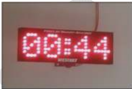
"Turn-Out timers" are installed in each apparatus bay to remind responders of their performance.
