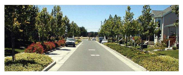
Example of a street meeting fire code and other operational needs, while limited to travel lane widths of 10 feet. By insetting parking, the built environment cue changes, altering driver behavior. Elimination of center lane lines, vertical walls of trees and ground cover also add to neighborhood friendly driving behaviors.
