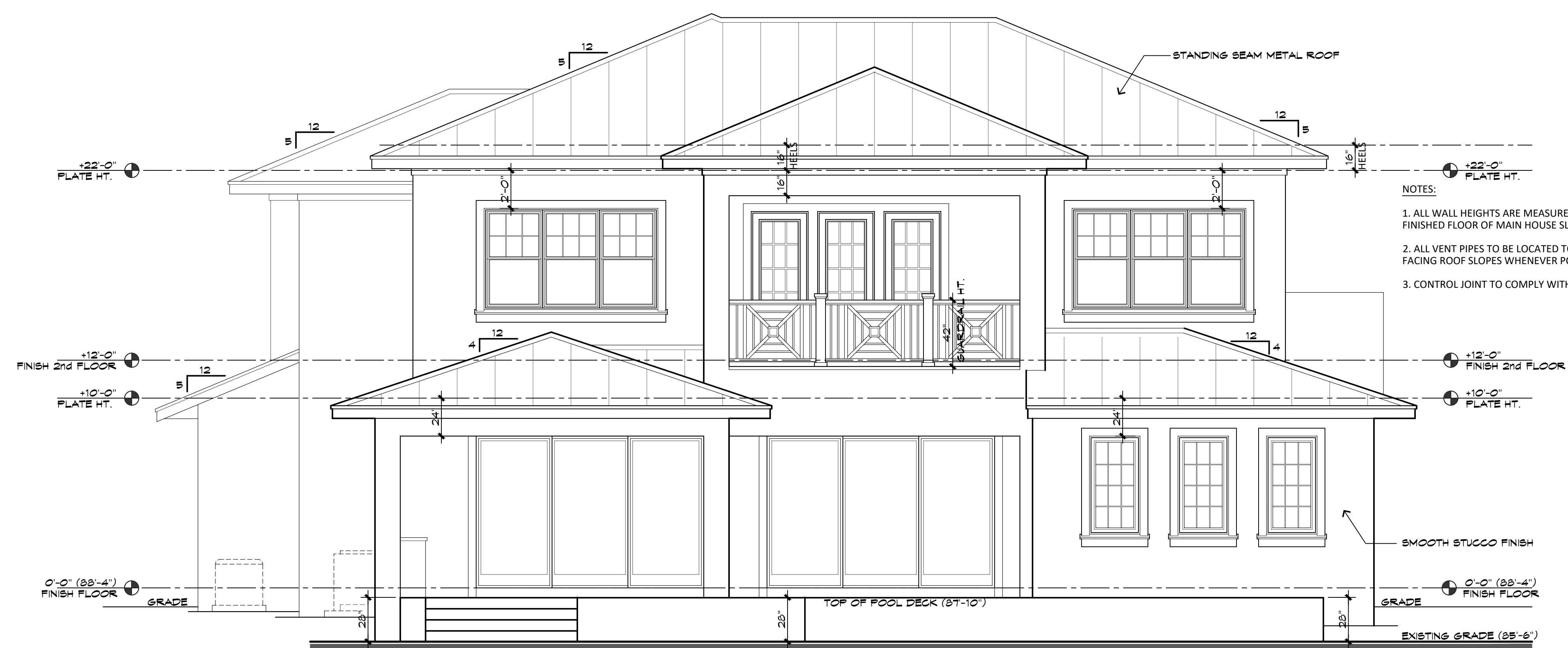
REAR ELEVATION scale: 1/4" = 1'-0"
