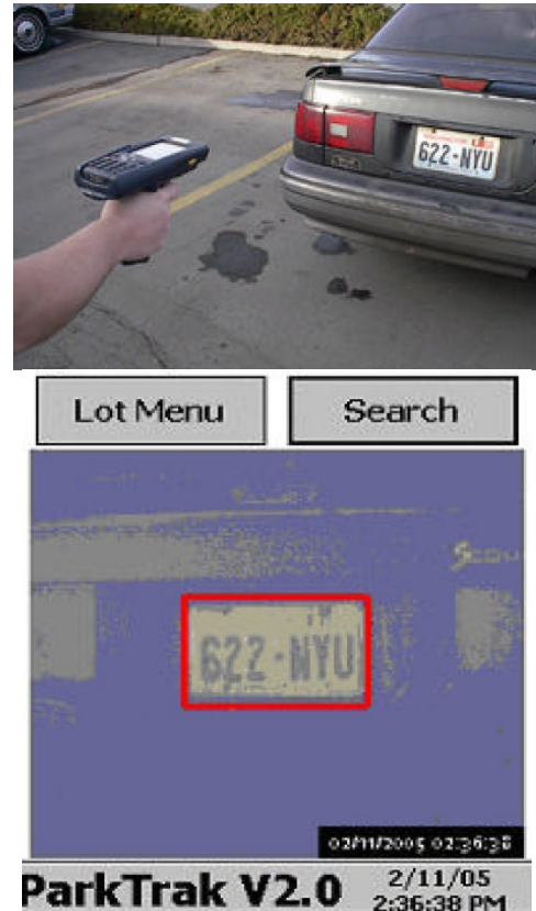
Figure 9: Electronic Handheld with License Plate Recognition Technology
