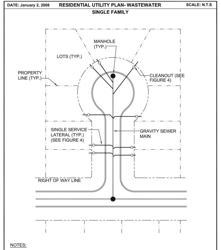
1. EACH SERVICE SHALL TERMINATE AT A CURB STOP(S) WHICH SHALL BE BURIED APPROXIMATELY 3" BELOW FINAL GRADE AND CLEARLY MARKED WITH A 2" X 2" X 18" STAKE AND PAINTED WITH THE COLOR OF THE PROVIDED UTILITY SERVICE AND LABELED WITH LOT NUMBER IT SERVES.
