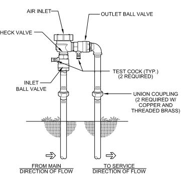
A PVB SHALL BE INSTALLED A MIN. OF 12' ABOVE THE HIGHEST POINT OF USE IN DOWN STREAM PIPING SUPPLIED BY OR FROM THE ASSEMBLY
